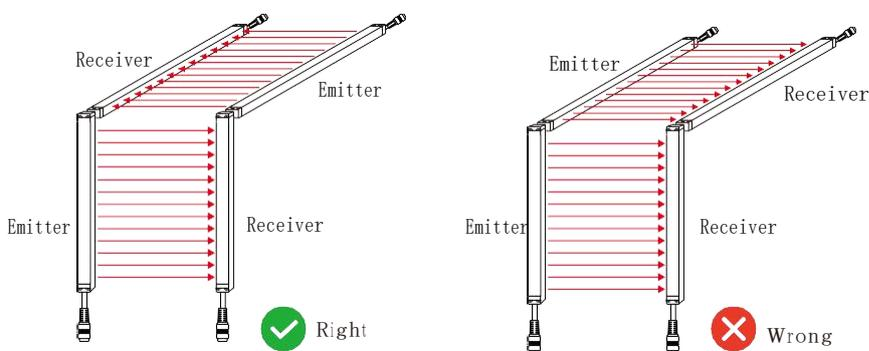
Note: In the use environment of L-type or concave-type, the adjacent safety grating transmission and reception need to be installed crossly.
