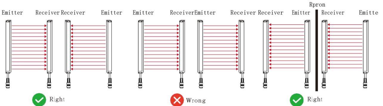
Note: If the distance between multiple sets exceeds the farthest distance of the safety grating, this installation scheme can be ignored.
