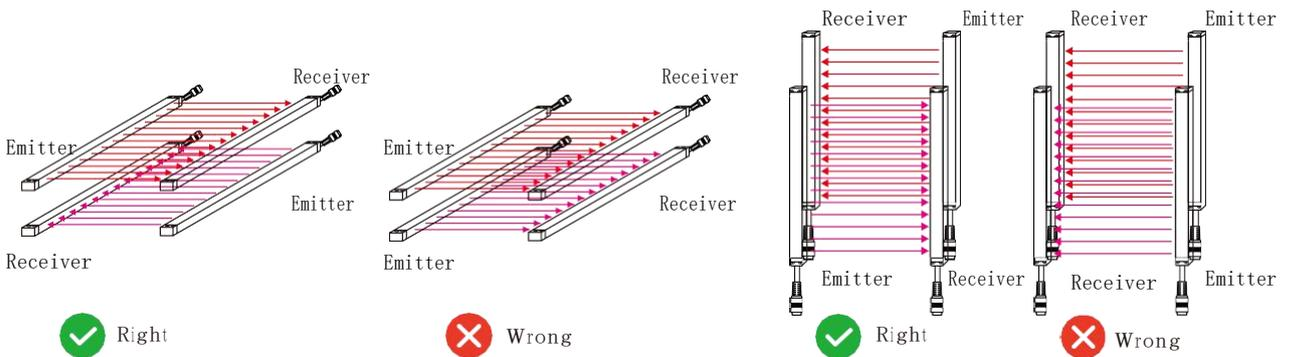
Note: Multiple sets are used to ensure that the adjacent two sets of safety gratings are installed cross-receiving and transmitting as far as possible from the same direction of the safety grating.
