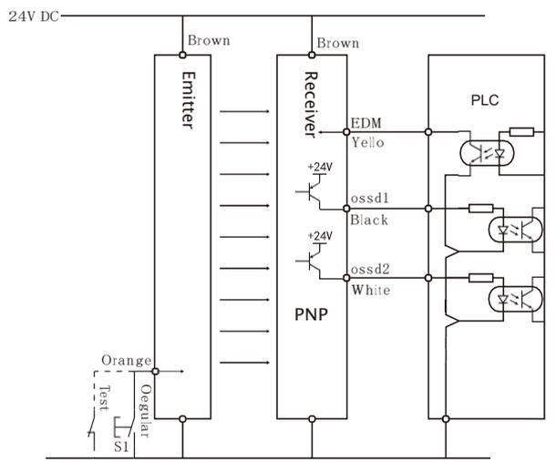
The Reference Program of SLC (NPN Type) Connection with PLC
